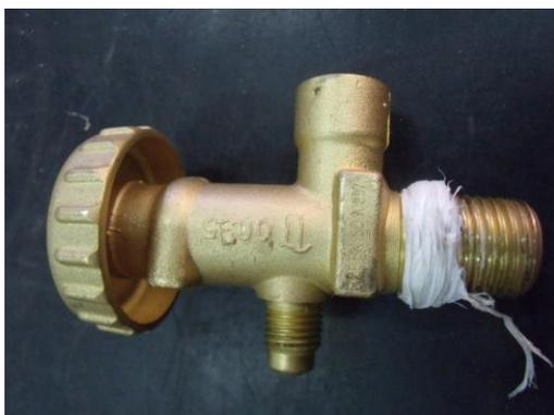
The Teflon seems not applied over the thread of the valve.
